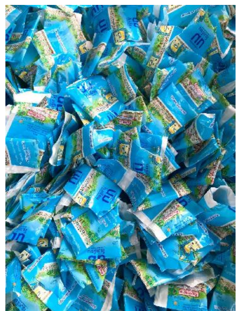
Packaging for milk is preferred to other types of plastic bags because it can make the paver tougher
