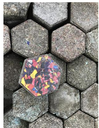
The recycled blocks are more durable and lighter-weight than normal pavers
